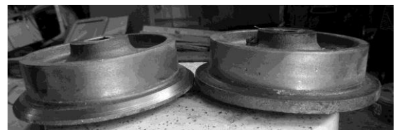
Flange before (right) & after (left).
